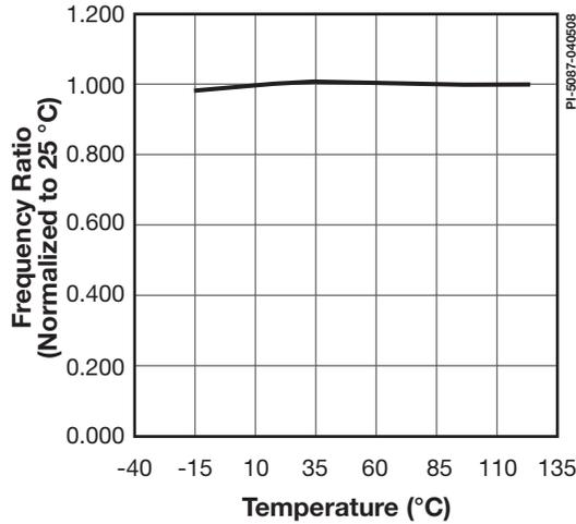
Figure 12. Frequency Ratio vs. Temperature (Constant Current).
