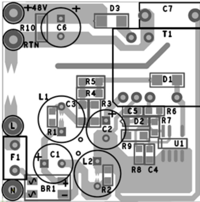
Figure 5. PCB Layout Example using SO-8C Package.
