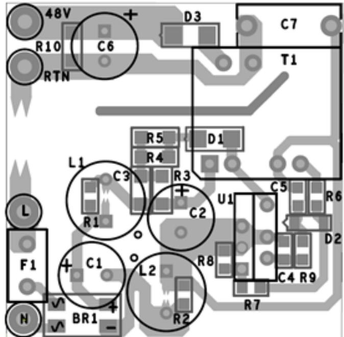
Figure 6. PCB Layout Example using eSIP Package.
