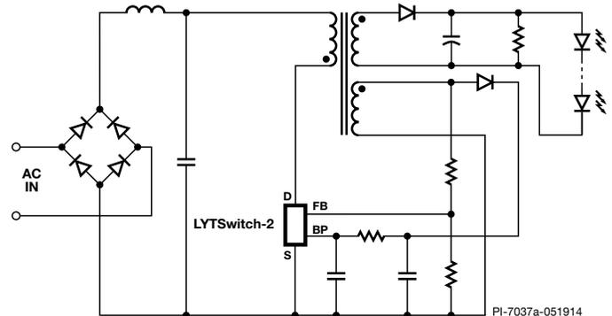
Figure 1. Typical Flyback Implementation – Not a Simplified Circuit.
