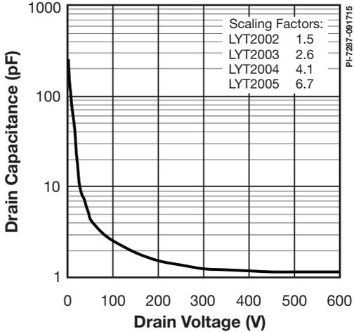
Figure 18. C<sub>oss</sub> vs. Drain Voltage.
